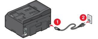
Connect the power cord to a properly grounded electrical outlet that is near the product and easily accessible.
